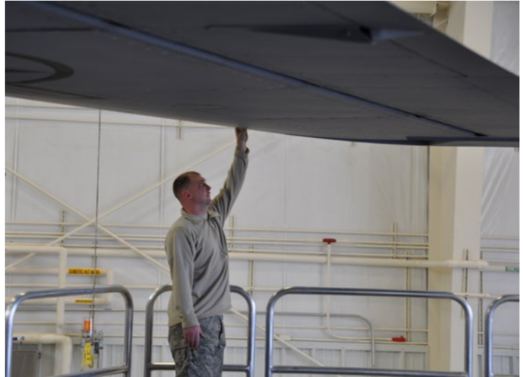
Master Sgt. Jason Lawson, 507th Air Refueling Wing maintenance squadron checks the distance between the new KC-135 maintenance platforms and the wing of a KC-135. The new platforms are expected to increase safety during Isochronal Inspections. (Photo by Senior Airman Mark Hybers)
